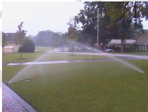
Figure 4-5. These two rotor applicators have overlapping radius of throw to get a more even broadcast application of the irrigation water.
